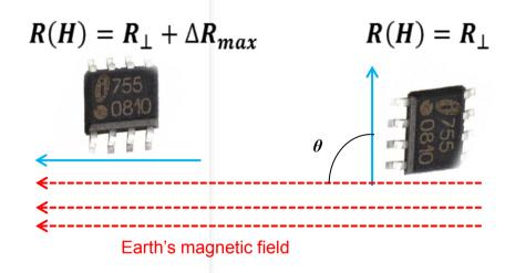
an Anisotropic Magnetic Resistive (AMR) Sensor
