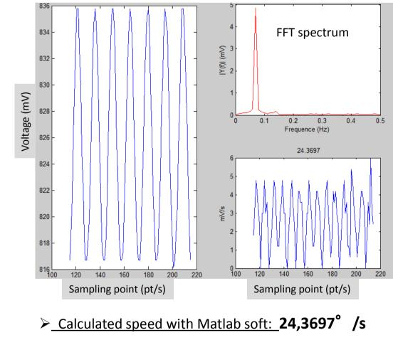
Servomotor speed: 20° /s
